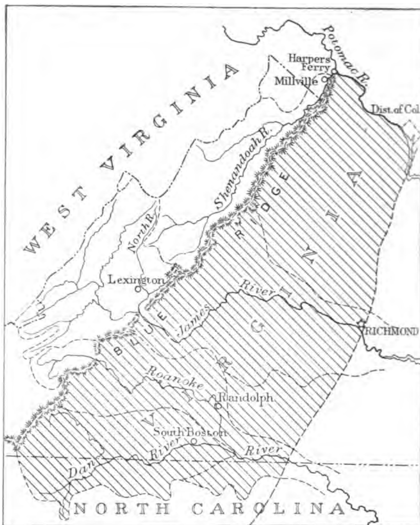
FIGURE 1.—Map showing geologic character of the drainage basins of Shenandoah, James, Roanoke, and Dan rivers. The shaded portion represents the area of crystalline rocks; the unshaded portion, sedimentary rocks. Dash lines represent limits of drainage basins.
